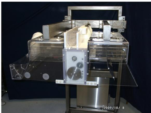
Depending on the powder's properties, the result can be a gravity-driven uniform deposition onto the product for the large particle powders like sugar and cinnamon. Very fine cohesive powders can be made to produce a rather incredible "smoke-like" dispersion which is introduced into the very efficient Terronics electrostatic powder deposition system gently drawing this fine material onto the food product.
